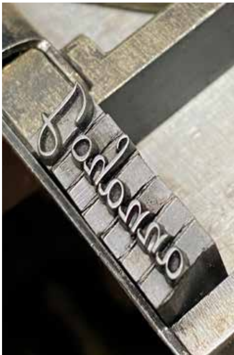
Lead type for printing on an 1880 platen press
